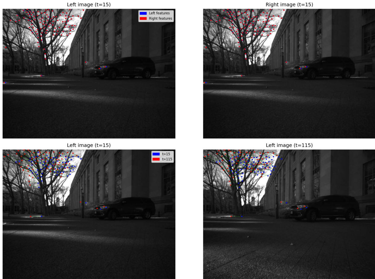
Fig. 2: Task 2: Feature detection and tracking on dataset02. Top: stereo matches at t = 15 (blue = left camera, red = right camera). Bottom: temporal tracks from t = 15 (blue) to t = 115 (red). Green lines show displacement in both rows.
